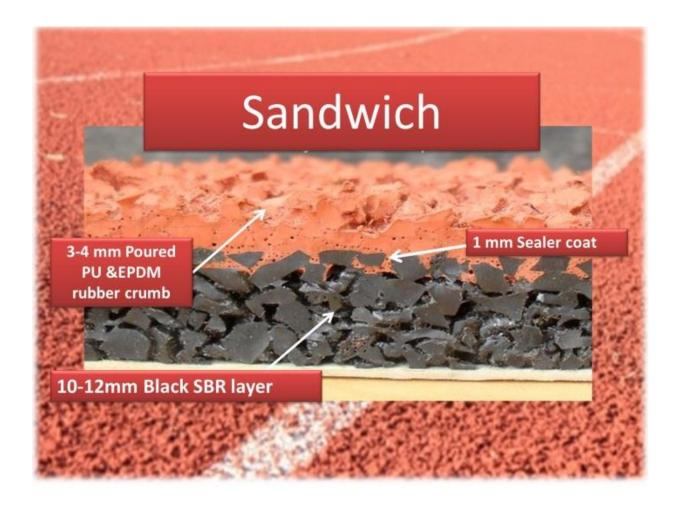
Often referred to as a 'sandwich' system, this hybrid system provides a non-porous elite level surface at a competitive price. This surface is constructed in two layers: A base layer made up of black rubber granules bound with polyurethane resin and a polyurethane flood coat combined with an EPDM surface dressing. As this type of surface is impermeable to water it relies on a fall in the track to a perimeter drain to keep the running surface free of surface water.
