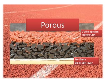
The system is made up of two layers: a sub base made up of black rubber granules bound with polyurethane resin, and a spray finish of coloured EPDM (rubber) granules and pigmented polyurethane.
